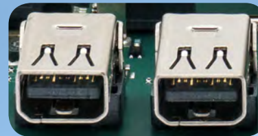
Dual-Mini-DP-Support Single Display Max. 4096 x 2160 @ 60 Hz
